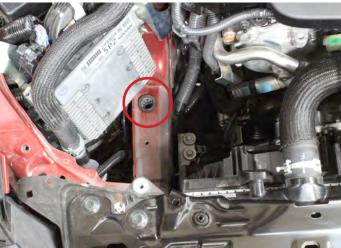
10. Remove the MAF housing from the rear section of the OEM air box. The Phillips head screws and O-ring will not be reused.
