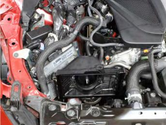
06. Disconnect the OEM coupler from the rear section of the air box and remove the air box.
