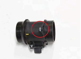
TECH NOTES: Pem nuts are often referred to as clinch style captive nuts. They press into a drilled or punched hole with an arbor press or similar pressure tool. In this case, as we're installing it into a plastic material, a pair of pliers will do the trick. Below is a close up of the Pem nut supplied. You can see the knurled area that is slightly tapered. This will lock the nut in place after it is pressed into the MAF housing.
