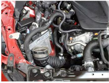
08. Disconnect the PCV hose from the OEM coupler. Only disconnect the small clamp at this time. Completely remove the OEM coupler.
